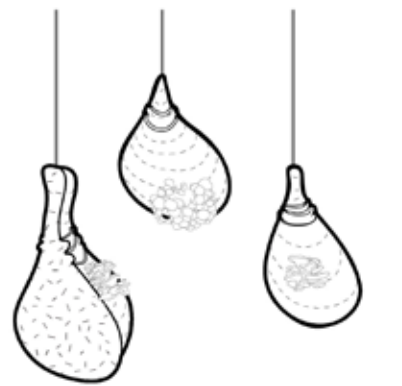
PRESSED MYCELIUM FILTER process | formed through pressing mushroom root mix into form-work and air drying or baking intent | roots can filter CO2 from air [biodegradable, placed in bag to serve as mass growth surface, where the carbon from the CO2 is then absorbed in the shell-growth process]
