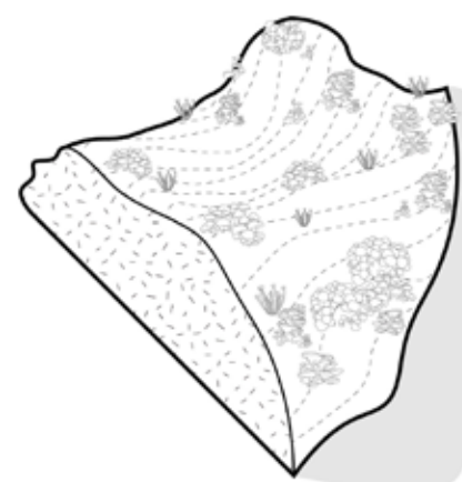
MYCELIUM WRAP BANK process | substrate + spores wrapped in plastic, punctured to allow for mushroom growth
