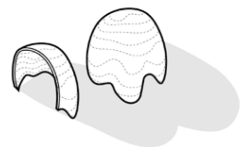
PRESSED HARVESTING STOOL process | formed through pressing mushroom root mix into form-work and air drying or baking intent | seating + stepping stones through mycelium rooms
