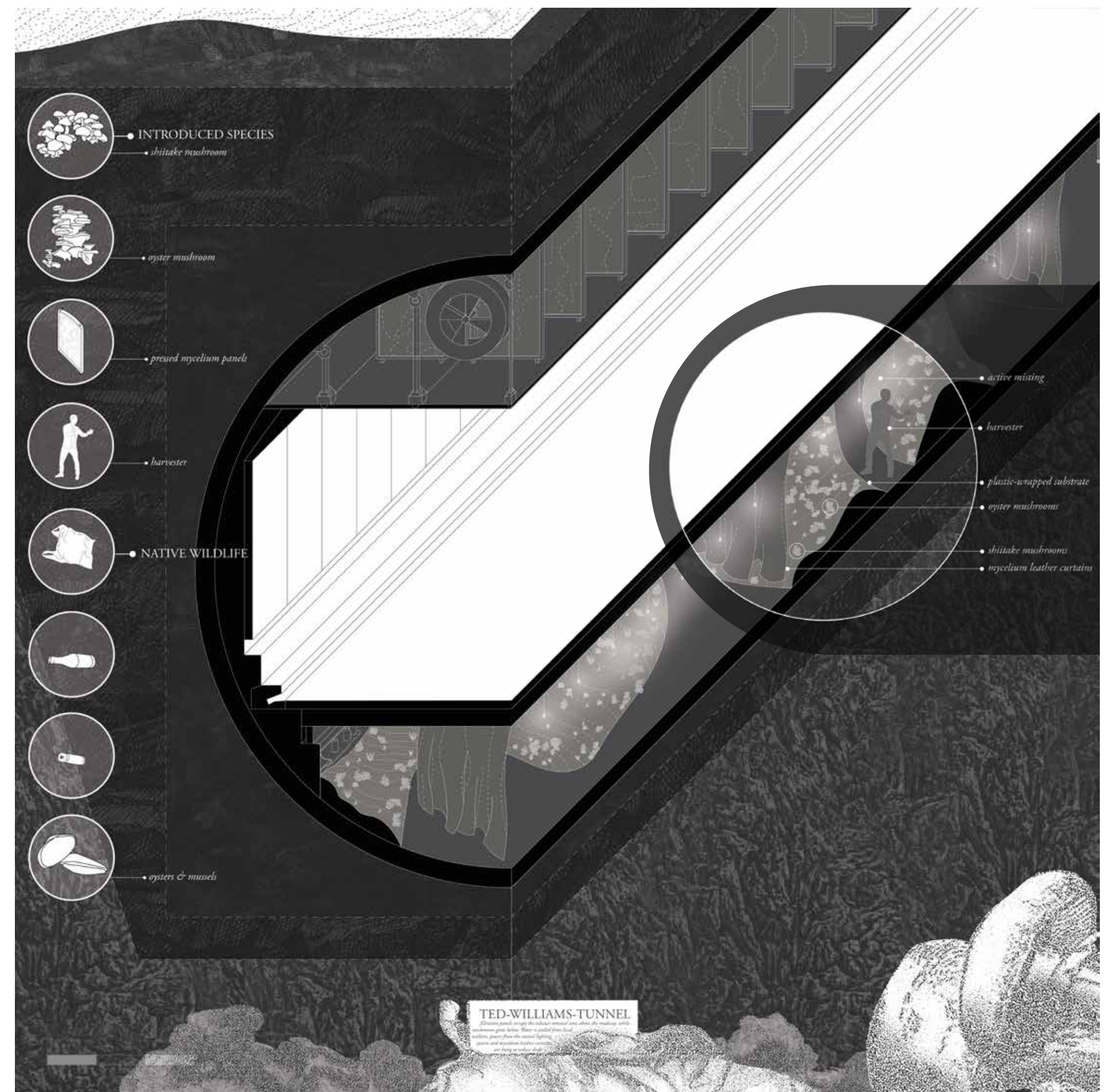
(above) TED-WILLIAMS-TUNNEL. filtration panels occupy the exhaust removal area above the roadway, while mushrooms grow below. Water is pulled from local utilities, power from the tunnel lighting, and mycelium leather curtains reduce draft.
